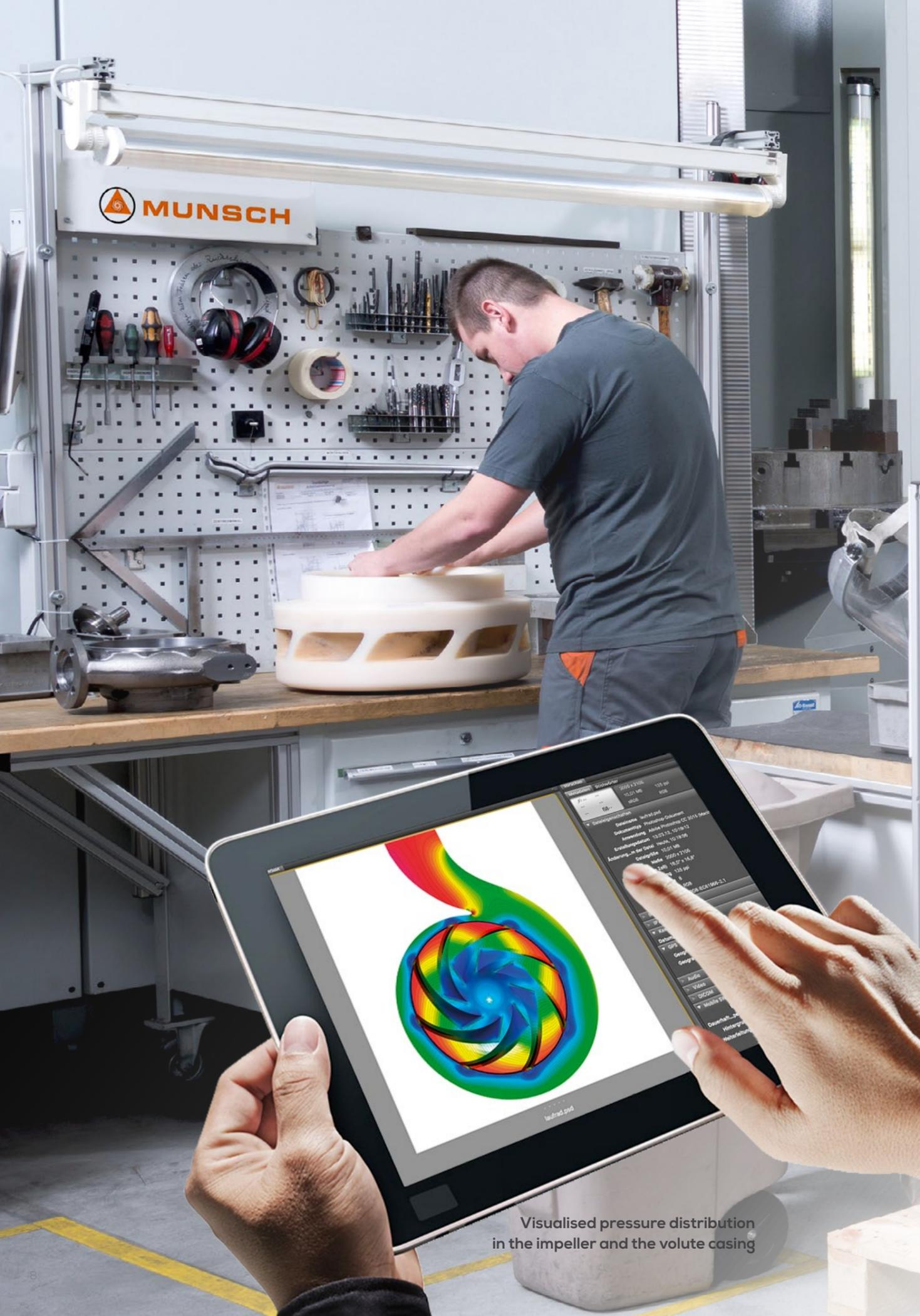
Visualised pressure distribution in the impeller and the volute casing
