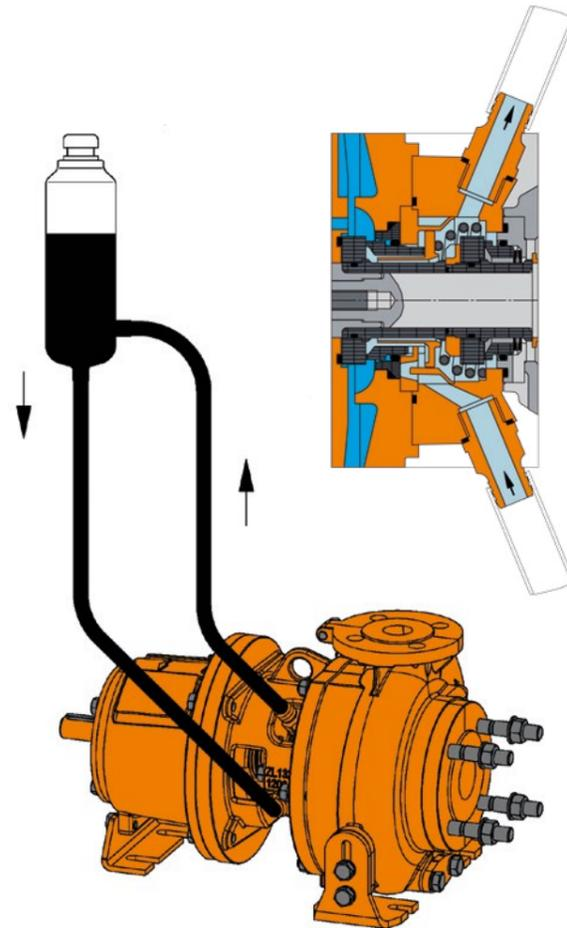
Pump with quench tank
