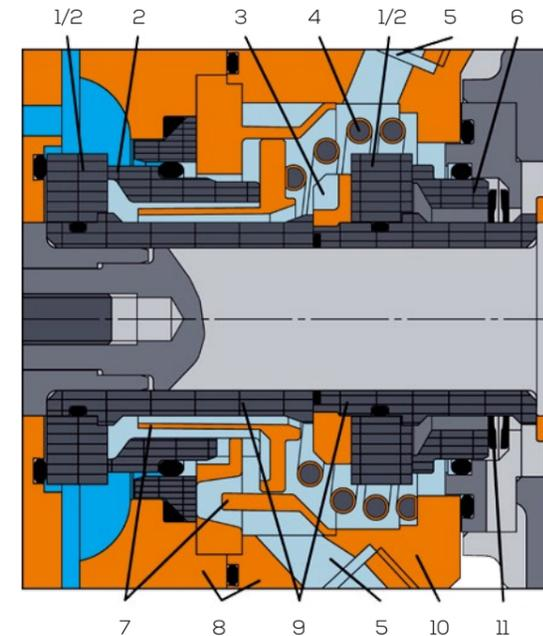
1. Product- and atmosphere-side rotating seal rings are of identical design and interchangeable.
