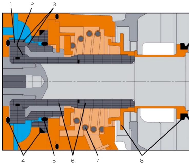
1. The rotating stationary seal ring design with a larger outer diameter effectively counteracts edge pressure.
