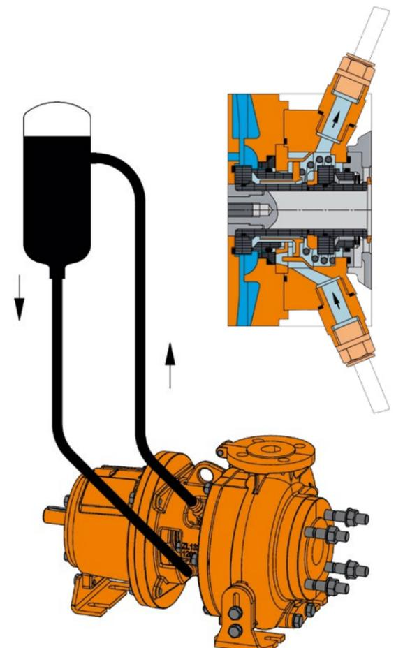
Pump with thermosyphon vessel
