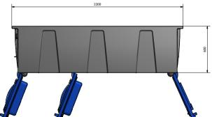
NOTE:-IF TANK HAS A SIDE MANWAY BOLTS TO BE TIGHTENED USING TORQUE WRENCH SET AT 95Nm CUSTOMER TO RE-TORQUE DURING ON SITE HYDROSTATIC TEST
